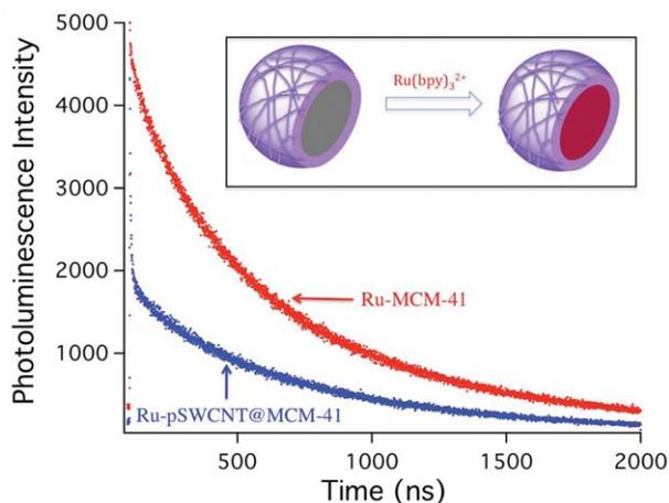
**Fig. 5** Time-resolved photoluminescence decay for Ru(bpy)<sub>3</sub><sup>2+</sup> in MCM-41 (—) and pSWCNTs@MCM-41 (—). The samples were excited at 444 nm and emission was recorded at 620 nm.
