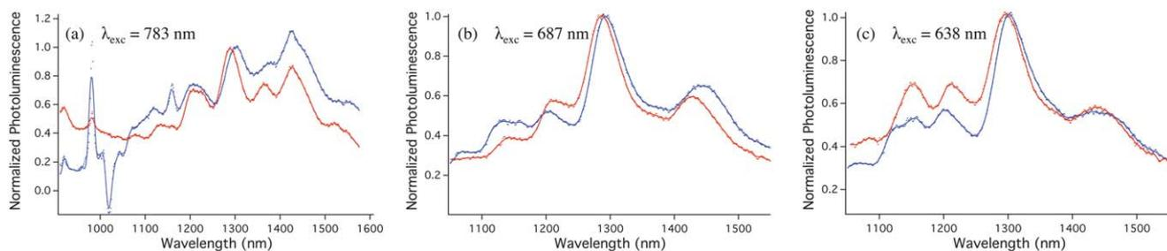
**Fig. 4** Photoluminescence spectra of vpSWCNTs@MCM-41 0.67% (w/w) (—) and SWCNTs dispersed in NMP (—).
