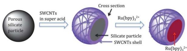
**Fig. 1** Pictorial representation of the deposition of SWCNTs onto the external surface of a porous silicate material and the subsequent loading of the photoactive molecule  $\text{Ru}(\text{bpy})_3^{2+}$  within the pores of the silicate particle.
