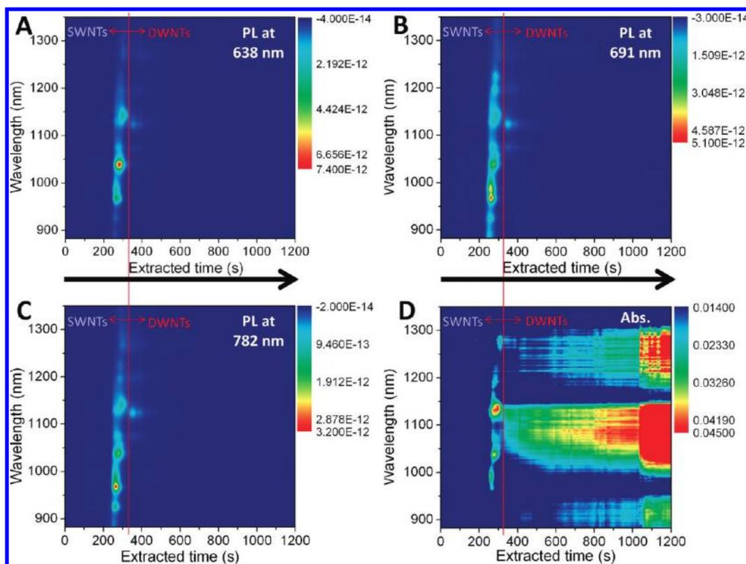
**Figure 2.** PL maps from separated SWNTs and DWNTs excited with: (A) 638, (B) 691, and (C) 782 nm lasers. X-axis is time frame in seconds, Y-axis is the emission wavelength in nm, and (D) shows the absorption map with the same time frame. The color represents signal intensity in both PL (nW/cm<sup>2</sup>) and absorption spectra using the presented color scale.
