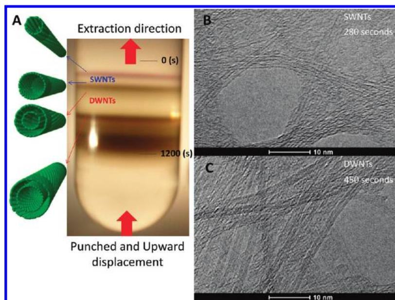
**Figure 1.** (A) Digital image of separated layers of CNTs using DGU method. All layers are labeled, and the time scale shown in the middle is corresponding to the time in spectral plots. After 1200 s, all layers of nanotubes are extracted from the centrifuge tube. (B) TEM image of samples extracted at 280 s, in SWNT region. (C) TEM image of samples extracted at 450 s, in DWNT region.
